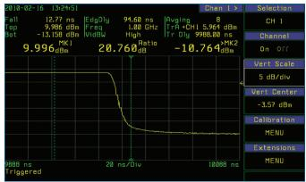
The markers show that the break point occurs approximately 20dB below the top of the pulse, equating to about 1% of the pulse power. With this in mind, it should be noted that a pulse fall time is normally measured between the 90% and 10% levels, and so will not be influenced by this characteristic.
