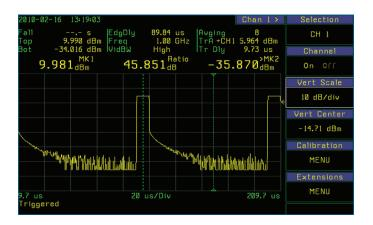
This is the normal response of many diode sensors, not only Boonton's, and carrying out the measurement in a logarithmic dBm scale results in an exaggerated tail. This may appear significant, but is in fact negligible.
