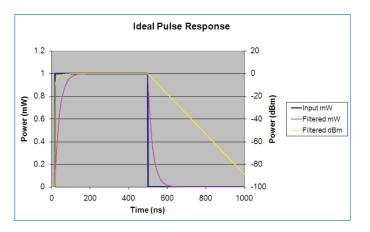
The leading edge compression and trailing edge expansion is very clear when the log scale is used. In linear mW, the leading and trailing edges appear symmetrical.
